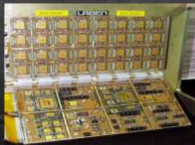
Pixels CaeSium Iodide Telescope (8 x 512 pixels)
