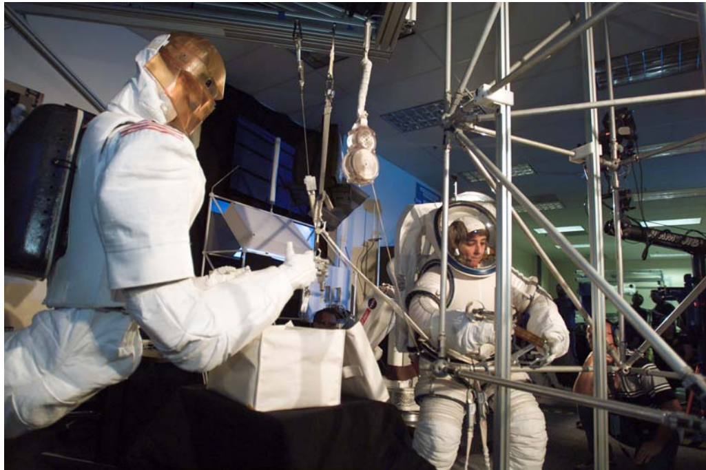
Figure 5: Astronaut and Robonaut prototype working together in truss construction in Earth laboratory (courtesy of NASA)
